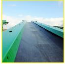
Stockpiling Ability At 40" wide and 65' long, the conveyor is able to handle large amounts of product.
