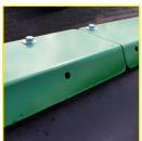
Enclosed Conveyor Sides For safety and efficiency, the conveyor sides are enclosed with flashing.
